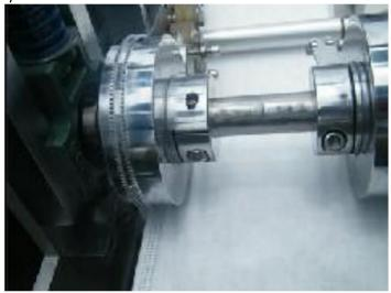
5.3.2. Imported ultrasonic transducer, 20K international frequency standard, output is more powerful and stable; coupled with two sets of ultrasonic system, effectively guarantee the welding quality of the product.
